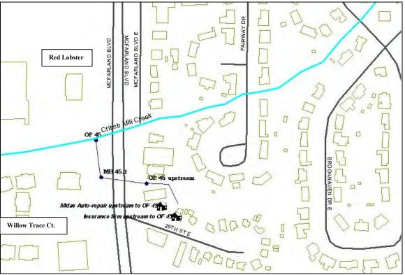
Figure 3. Drainage System Associated with Outfall 45.
