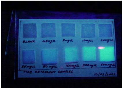
Figure 1. Standard Tide Optical Brightener Pads
